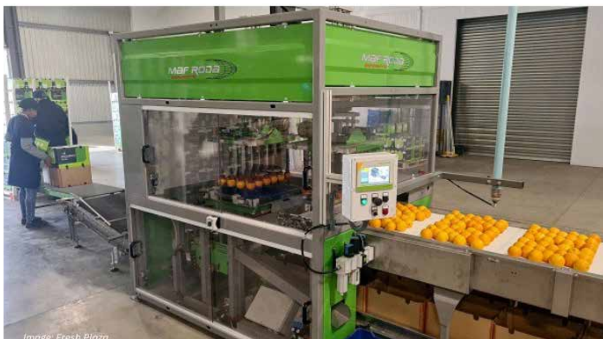
Figure 20: A Maf Roda V8 speed packer with Jumble Filler Combo in operation. Source: 2 fruit plaza, online magazine.
