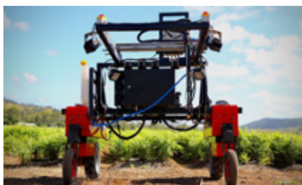
Figure 22: Mechanical weeding using motorized finger weeder (Image credits: Left, Cioni and Maines, 2010; Right, AgriFutures, Australia)
