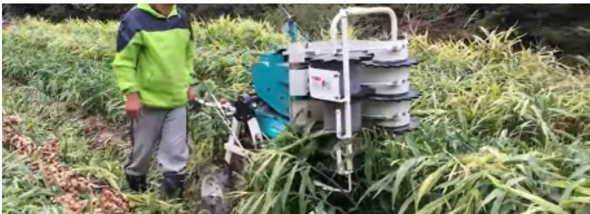
Figure 55: Mechanical trimming of ginger placed in lined field trays (Image credit: Discover Agriculture )
