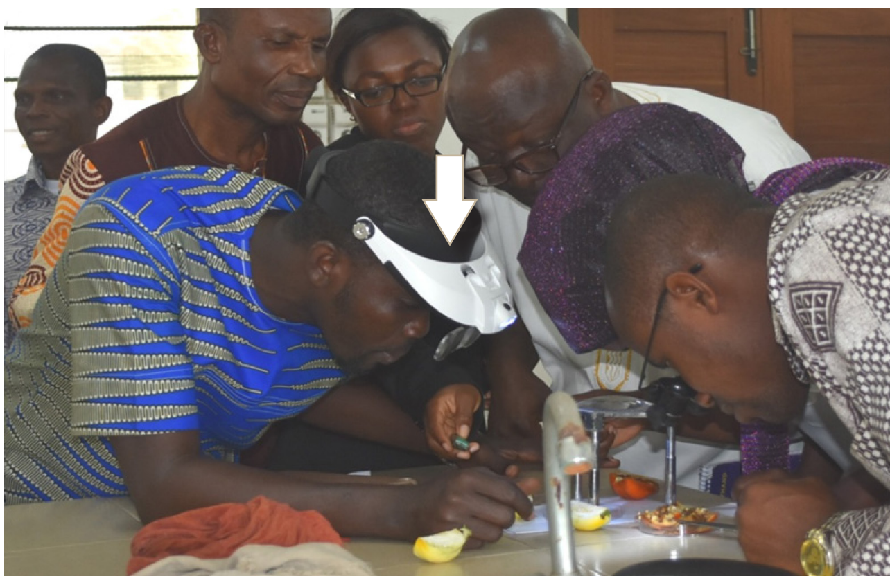
Figure 13: Using the head visor, fitted with a magnifying lens, for inspecting the presence of quarantine pest in produce. (Photo by KO Fening, University of Ghana) (see arrow).
