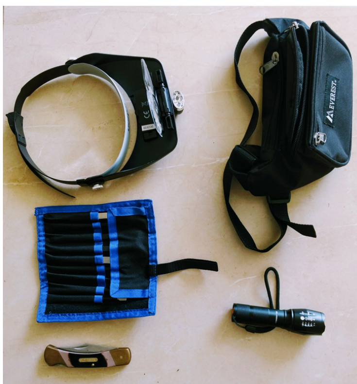
Figure 14. Recommended inspection tools (head visor fitted with a magnifying lens, inspection tools bag, forceps and knife or dagger and touch light above), recommended for the pack house to detect pests in commodity for export. Photo by KO Fening, ARPPIS, University of Ghana.
