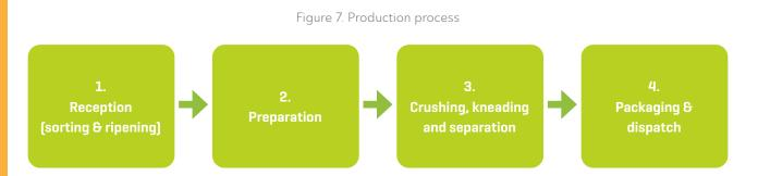
In *step 1, reception*, avocadoes are received at the factory and sorted to ensure that the quality standards set for the product are met. Ideally, the avocadoes will be ripened after reception. A ripening room would be used and the process might include the use of ethylene.
