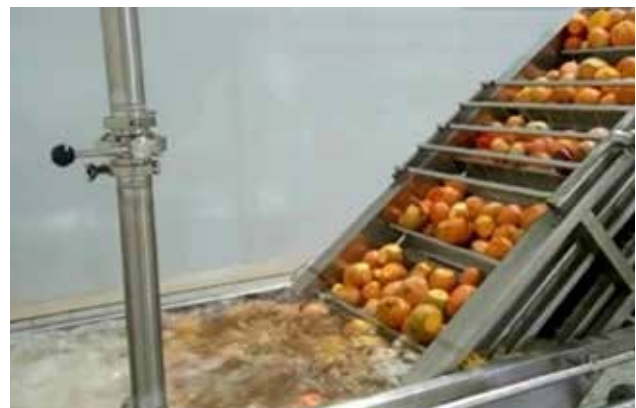
Figure 13. Elevator that lifts mango for sorting
