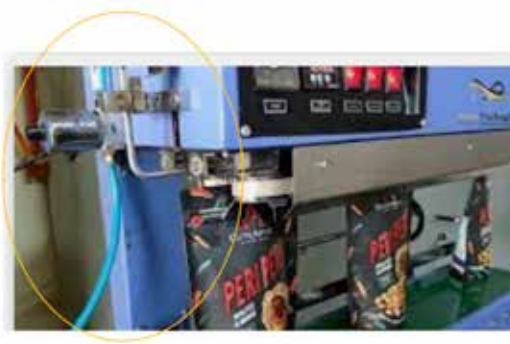
Figure 19. Form-fill-and-seal machine using a nitrogen flusher
