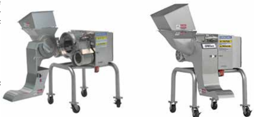
Figure 14. The Urschel Diversacut Sprint, suitable for cubing, slicing and pulping a large variety of fruits and vegetables Source: Urschel.
