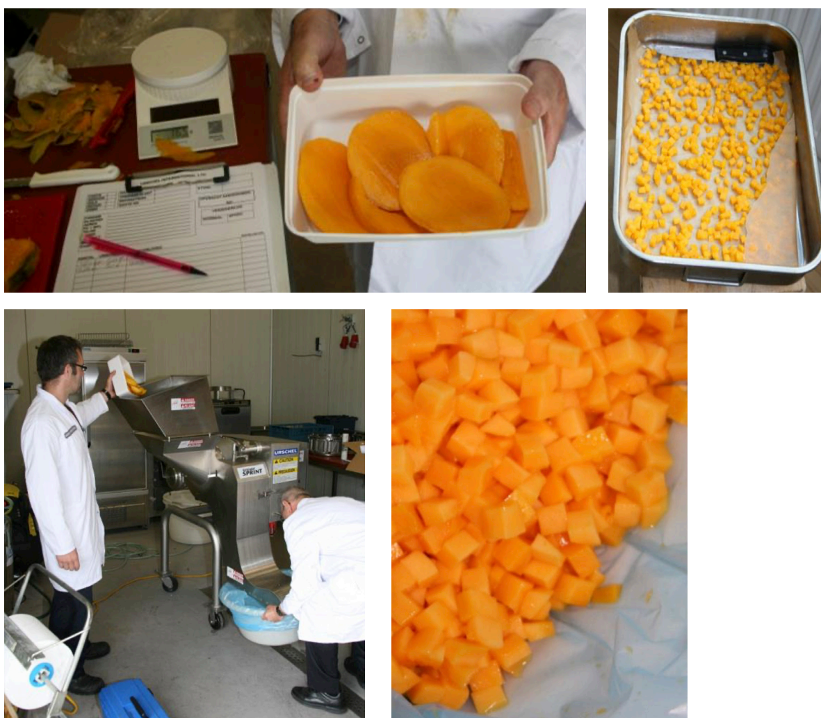
Figure 17. Production of IQF samples: cutting and weighing of the cheeks (top left), cubing by machine (bottom left), collection of freshly diced cubes (bottom right) and freezing of the cubes (top right) Source: authors from factory visits.
