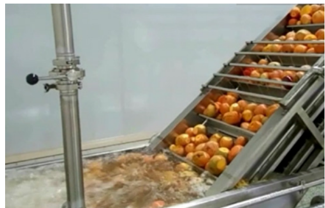
Figure 13. Elevator that lifts mango for sorting
