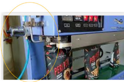
Figure 19. Form-fill-and-seal machine using a nitrogen flusher
