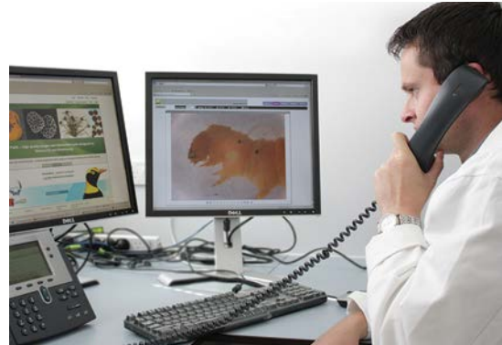
Figure 28: Specimens under the USB microscope may be shared with an expert via video software. In this case the conversation between the laboratory and the expert is over the telephone
