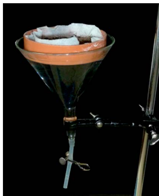
Figure 16: Modified Baermann funnel for extracting nematodes from plant material or soil
