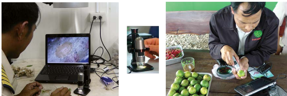
Figure 29: Left: A USB microscope captures images to a PC at a border inspection point and can be shared with remote specialists via web collaboration tools such as Skype. Centre: A 20–200× magnification USB microscope. Right: A Border Inspection Officer examines pests and captures images using a USB microscope
