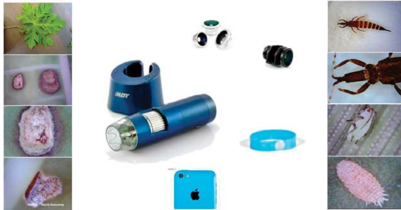
Figure 30: Centre: Various simple attachments enable mobile phones to capture highly magnified images of pests, which can be shared and discussed with communities via cloud networks. These communities can include local or regional NPPOs. Side images taken with the Hot Electronics wireless microscope and mobile phone. Left side images of papaya brown spot. Right side images show range of magnifications achieved with the wireless microscope
