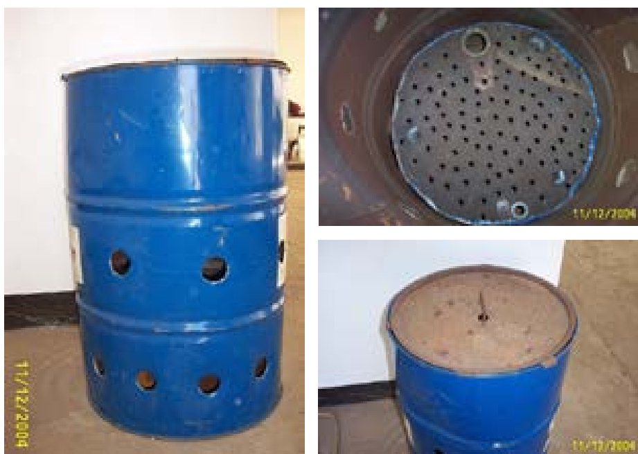
The incinerator container, the base grid and cover (Photos A. Diouf)
