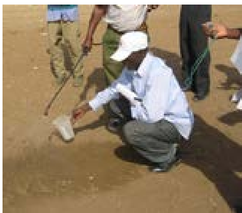
Measuring the output of a nozzle into a graduated container, measuring the time with a chronometer (Photo B. Schiffers)
