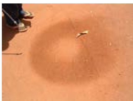
Trace left on ground by a hollow cone nozzle. The jet clearly forms a hollow cone. The finest droplets are at the exterior of the jet and are carried by the wind (drift). This type of turbulence jet is well suited for fungicide treatments as the fine droplets can adhere to the inner face of leaves. (Photo B. Schiffers)
