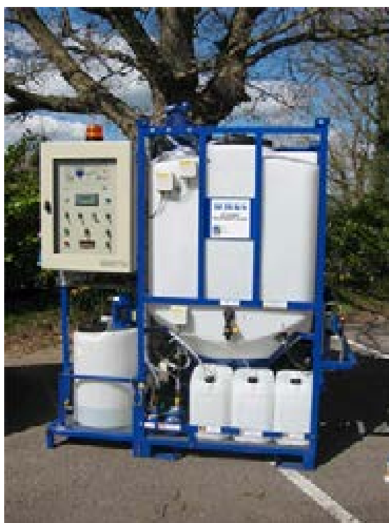
For the treatment of plant health product effluents from post-harvesting treatments, the SENTINEL device designed by WMEC (UK).
