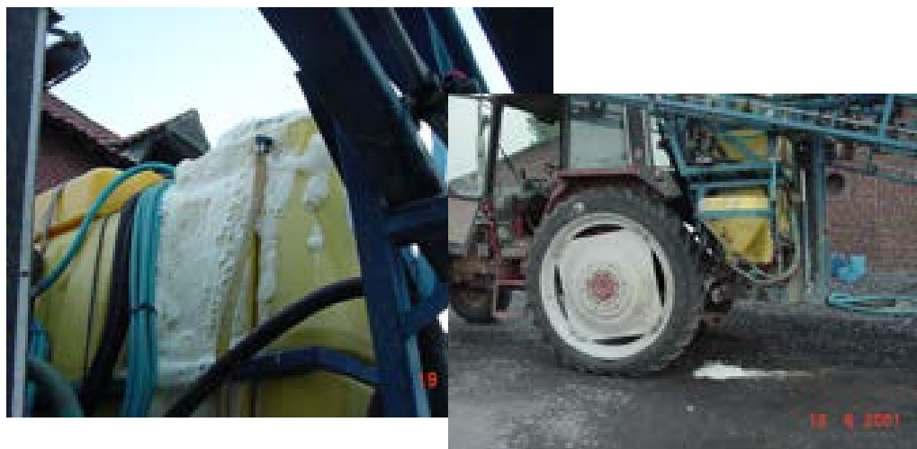
Overspill of the tank and leaks during filling (Photos Phytophar).
